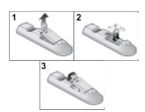
**NOTE:** Remove batteries from remote control when it is not to be used for a long period. Otherwise it can be damaged due to any leakage of batteries.
